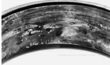
Adhesion on ball bearing
