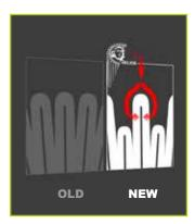
Particularly under high dynamic load conditions, the special geometry prevents the pleats becoming compressed and this reduces the differential pressure
