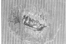
Surface fatigue on ball bearing
