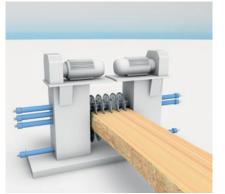
Saw units with single-blade adjustment make it possible to change the cross-section extremely fast. Hydraulic cylinders control the saw blades and Micropulse transducers reliably and accurately return the position. As a result, using them supports optimum exploitation of the wood.
