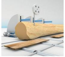
Vertical band saws adjust to maintain the desired board thickness after each cut. Micropulse transducers are excellently suited to configuring these settings quickly and with great versatility.
