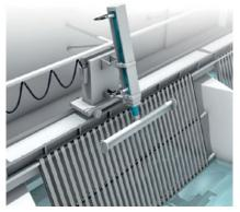
Floating debris at the infeed end of hydroelectric power plants causes efficiency loss and thus diminishes cost-effectiveness. The worst-case scenario could result in plant downtimes with high costs. With the highpressure resistant inductive sensors BHS, the end positions on the rake cleaner can be easily and reliably detected.
