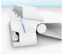
For paper production, hydraulic components must often work reliably under aggressive ambient conditions. For example, the headbox evenly applies the stock suspension on the wire mesh and thus influences the paper quality. Deckle plates and headbox bottom lip are hydraulically controlled. Precise position measurement systems in hydraulic cylinders ensure an optimal result.
