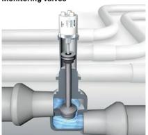
The highest safety requirements for emergency shutoff control valves require redundant systems. In compact redundant Micropulse transducer BTL 7, up to three independent measurement sections and three independent electronics systems are integrated in a rod. The robust, absolute position measurement system is freely configurable and easy to operate.
