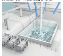
Compensation cylinders must maintain a specified tension of the marine riser and balance all fluctuations. To do so, the hydraulic cylinders are attached between tensioner ring and rig and equipped with position measurement. These smart hydraulics level the sea movement and ensure continuous tension of the production riser, independent from the upward and downward heave of the floating drilling rig.
