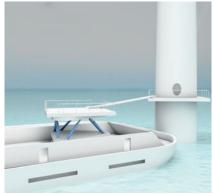
Security on the sea: Even with swelling, people from the supply vessel can safely reach the platform or the offshore wind power plant.
