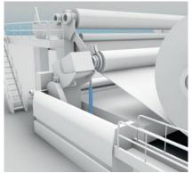
Produced paper is wound up around large rolls. At high production speeds, these rolls grow very fast and become extremely heavy. The most up-to-date hydraulic and position measurement technology ensures the best possible winding process. Micropulse transducers BTL that are securely packed in the hydraulic cylinder report the position.
