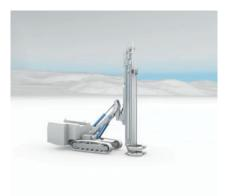
Always know where the driller is: When searching for new raw material supplies, soil samples are taken with mobile drillers to confirm potential deposits. Micropulse transducers BTL PF ensure reliability for the correct drilling depth.
