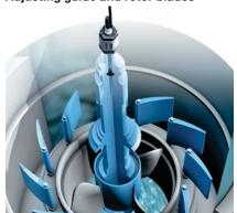
The guide and rotor blades on Kaplan turbines can be adjusted with help from BTL micropulse transducers. For example, a BTL profile controls the position of the guide vanes as needed. Another BTL integrated in the shaft ensures optimal adaptation of the impeller to the water volume.
