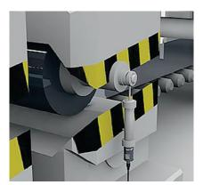
Micropulse transducers BTL guarantee high accuracy when winding the coils. The pressure roller is guided, for example, depending on the roll diameter.
