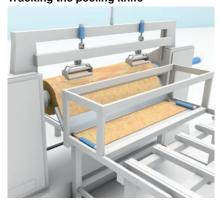
In veneer production, logs are peeled layer by layer. For an optimal result, contact pressure and the position of the peeling knife must be precisely controlled. This can only be successful through smart cylinders with a built-in position measurement system BTL.
