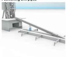
Pipehandlers take drill pipes out of the magazine and position them directly over the borehole. Quick and efficient drilling is thus ensured. Powerful hydraulics move the heavy rods with ease and bring them directly into place and position. Balluff position measurement systems are critical for prompt, correct positioning.
