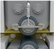
The roll gap can be set with high accuracy using the Micropulse transducer BTL in IP 69K during hot or cold rolling. The vacuum-sealed BTL does not require any additional protection for continuous water cooling of the rolling stand.
