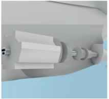
Variable pitch propellers bring critical advantages to the ship propulsion system. This is particularly worthwhile when there are frequently changing speeds, such as on ferries or cruise ships. Angle adjustment is hydraulic and is controlled by triple-redundant Balluff position measurement systems.
