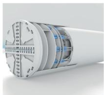
Tunnel boring machines remove rock centimeter by centimeter. Pushing cylinders, which continuously force the drill head into the rock, provide the strength needed for this. Micropulse transducers BTL correctly report the piston position and allow for a smooth drilling process.
