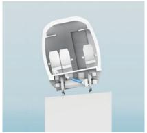
For shortened travel time and high cornering speeds, express trains are actively tilted up to 8°. Hydraulic cylinders with redundant Micropulse position measurement systems are used in inclination technology. For maximum passenger safety and optimal angles in every curve.
