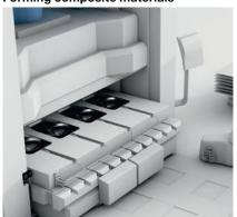
When producing components from carbonfiber-reinforced plastic (CFRP), the carbon fibers that are woven to mats are pressed into shape under heat and pressure. In this process, they must be monitored and harden uniformly. Micropulse transducers ensure uniform pressure with every pressfitting process without being impeded by
