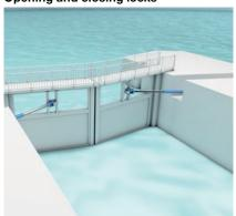
Hydraulic cylinders move the powerful gates of the large locks, which can take on enormous dimensions in seaports. BTL ProCompact HB transducers are used in hydraulic cylinders to exchange the water efficiently and monitor the position of the gates.
