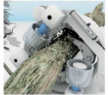
Sensors for debarkers are exposed to strong vibrations. Transducers in hydraulic cylinders monitor the piston position of the infeed unit. This enables logs of different thicknesses to be optimally fed.
