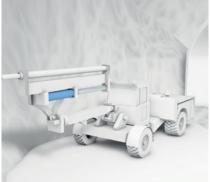
In raw material extraction, Micropulse BTL profile position measurement systems installed outside the cylinders monitor the drilling of the blast holes below ground. This is the only way that safe and reliable tunnel mining and efficient raw material excavation can be ensured.
