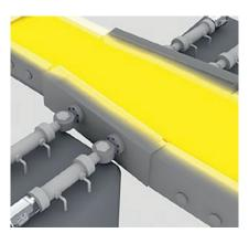
Micropulse transducers BTL in the hydraulic cylinder are ideal for positioning and guiding the slabs. They check for the correct configuration of the lateral guides and accompany the slabs on their path through the rolling stand. The large forces in the reshaping are reliably compensated for in this process.
