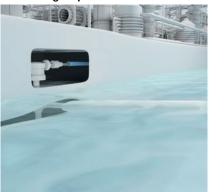
Particularly cruise ship passengers suffer from rough seas. Stabilizers are used so that the ship fluctuates less, which decreases ship movements. Depending on the position, the optimal fin angle is changed to keep the ship as vertical as possible in the water. The Micropulse transducer HB guarantees the correct adjustment.
