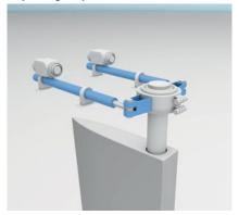
To keep a ship on target, the ship rudder must be continuously adjusted. This is successful with reliable and high-precision Balluff position measurement technology. Position measurement systems BTL rod (integrated in the hydraulic cylinder) and BTL profile check the rudder position from start to finish and allow for exact readjustment.
