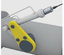
Micropulse transducers BTL are used for controlling flaps and valves on the blast furnace in order to regulate the supply and exhaust air during production of pig iron. Alternatively, standard inductive sensors BES deliver convincing performance. Additional security: A temperature sensor is integrated in the electronics head for all micropulse transducers BTL with a bus interface. This guarantees the correct temperature measurement.
