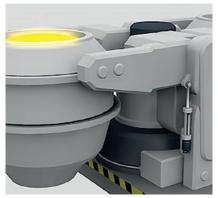
Ladles ensure replenishment of steel in production. Optimal control over the process and ensuring the addition of the correct quantity of steel in the continuous casting line is only possible through precise ladle movements. Micropulse transducers BTL7 (double and triple-redundant) provide absolute security and the best reliability for the continuous casting process.
