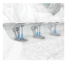
In mining, shields prevent rocks from falling in the working area and injuring miners. To support longwall mining, hydraulic cylinders are used. Micropulse BTL position measurement systems of the K series integrated in the hydraulic cylinders provide exact positioning and secure monitoring of the shields.
