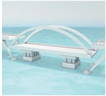
When building bridges, special heavy-duty cylinders carry out horizontal feed and vertical lifting motions to move the bridge elements, which weigh multiple tons. The Micropulse transducer rod CD is installed in the pressure area of heavy-duty cylinders and high pressure cylinders to position these extreme loads synchronously and with millimeter precision.
