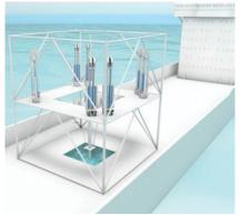
Wire-lines connect floating drilling rigs to the seabed. These are held under tension at all times to prevent damage. During swelling, tension is hydraulically adjusted to the clamping device. When this occurs, the piston position of the cylinder must be reliably reported back. Micropulse transducers BTL execute this perfectly.
